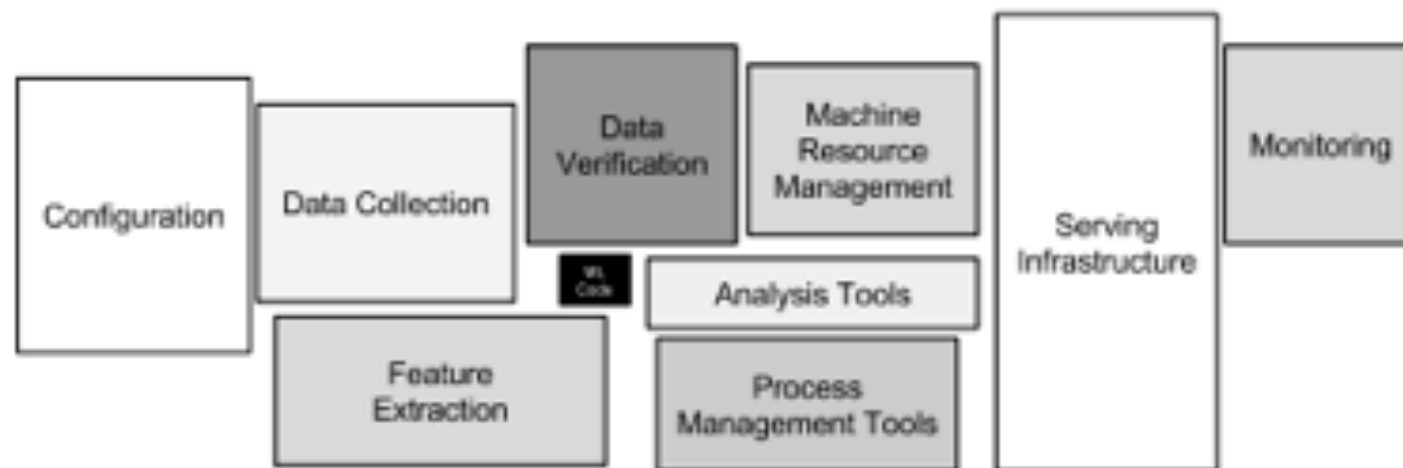
Figure 1: Only a small fraction of real-world ML systems is composed of the ML code , as shown by the small black box in the middle. The required surrounding infrastructure is vast and complex.
